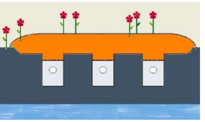
A capping fill drainfield is similar to a standard drainfield; however, the soil is manipulated to maintain adequate separation to the ground surface while allowing sufficient distance from:
